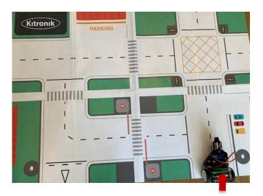
Step 5: Turn on the power button on the back of the Maqueen, robot and then press the **A button** on the BBC micro:bit board.
